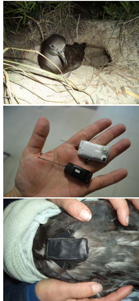
Figure 10. Photos of a shearwater and the GPS unit glued to the animal in the Pindai colony in New Caledonia (images: Karen Bourgeois)
