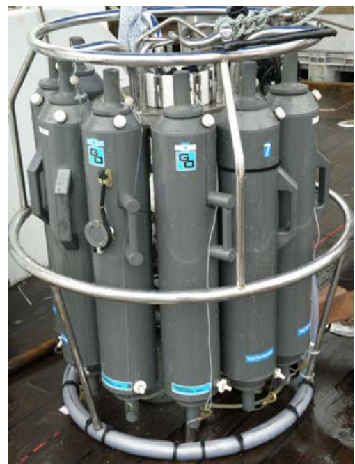
Figure 7. The rosette used on the RV Alis for water sampling (image: Florian de Boissieu, IRD).
