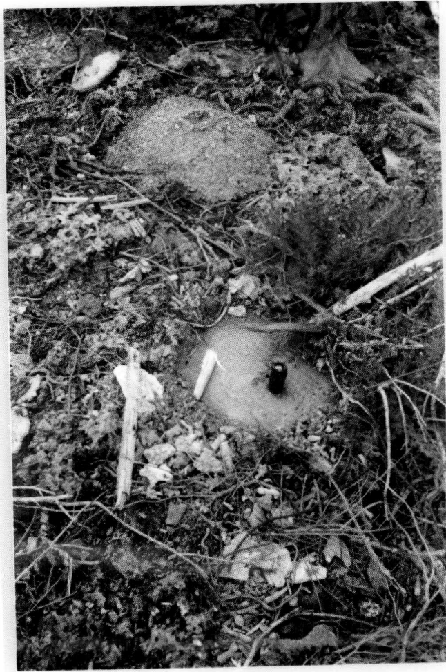
Illustration of bench mark 12.7.39 at centre top of photo. At this particular site there are five bench marks within a radius of about 5 metres.
