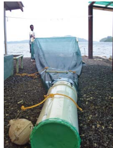
Figure 1. The crest net with a 320-mm PVC pipe fitted as a cod end.
