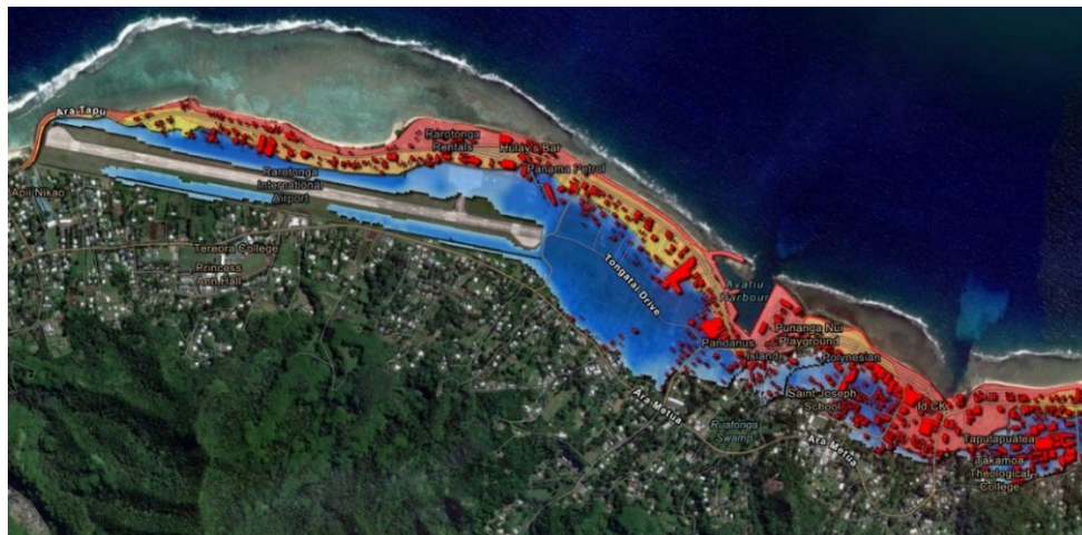
Map 3. One-in-100-year ARI for tropical cyclone events on the Avarua to Nikao coastline. 24
