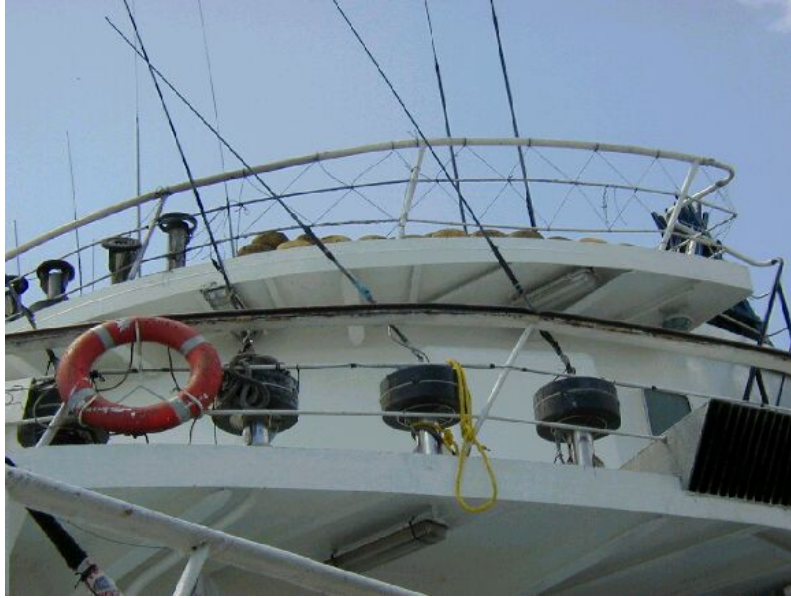
Figure 58. Inclined antennae on RDF buoys (photo D. Itano)
