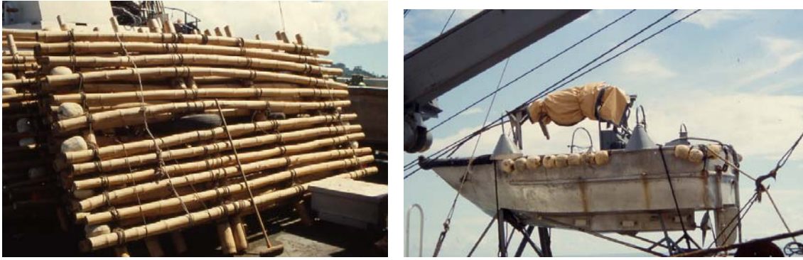
Figure 6. Bamboo raft style anchored payao tried in Fiji and a light boat used during pre-dawn sets.
