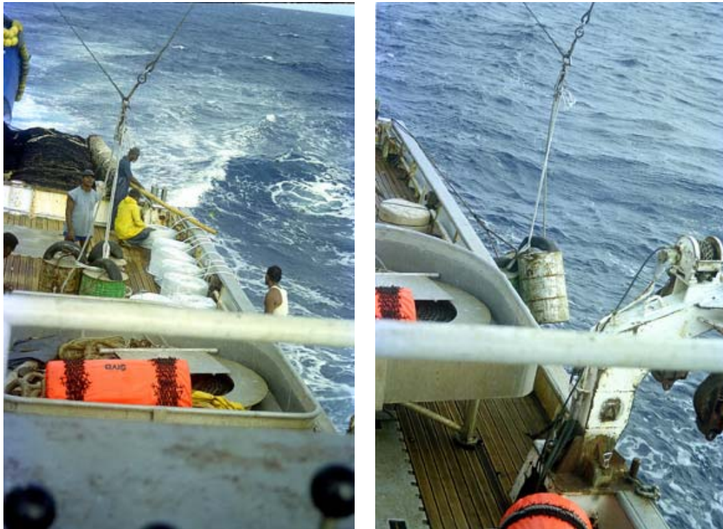
Figure 8. An NFD anchored FAD being set off the Solomon Islands with rope and anchors being set after the FAD float has been released (photos D. Brogan)
