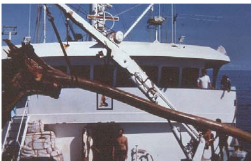
Figure 14. Recovering a natural drift log to use as a FAD and roping several natural drift logs together to form one large raft to aggregate tuna for purse seining (photos D. Itano)
