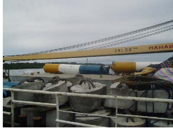
Figure 11. Philippine style cylindrical payao on station and a FAD tender vessel loaded with cement anchors and new FAD floats (photos S. Fukofuka)
