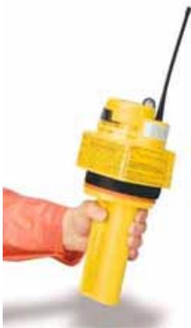
The GPIRB is the first of a new generation of emergency beacons. Global Position Indicating Radio Beacons combine the latest in GPS and 406MHz EPIRB (Electronic Position Indicating Radio Beacon) technology, and add extraordinary precision to your emergency distress signal. If you are a boater who operates offshore, this could be the best 'life insurance' policy you own.
