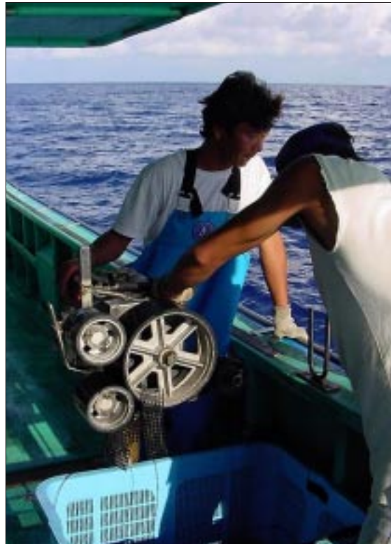
Electric hand reels for hauling droplines
