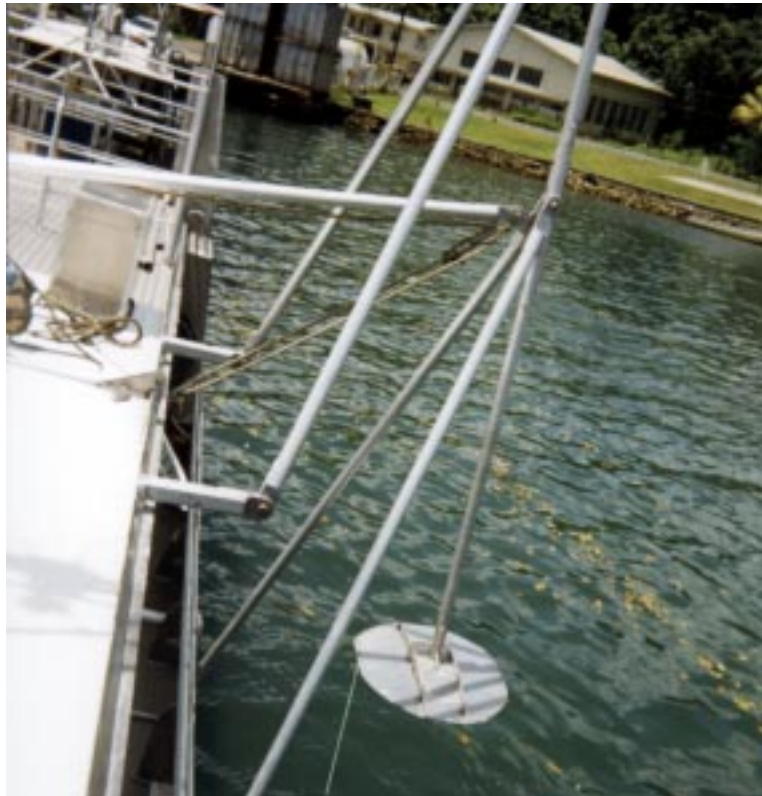
Figure 4: Flopper-stopper being deployed
