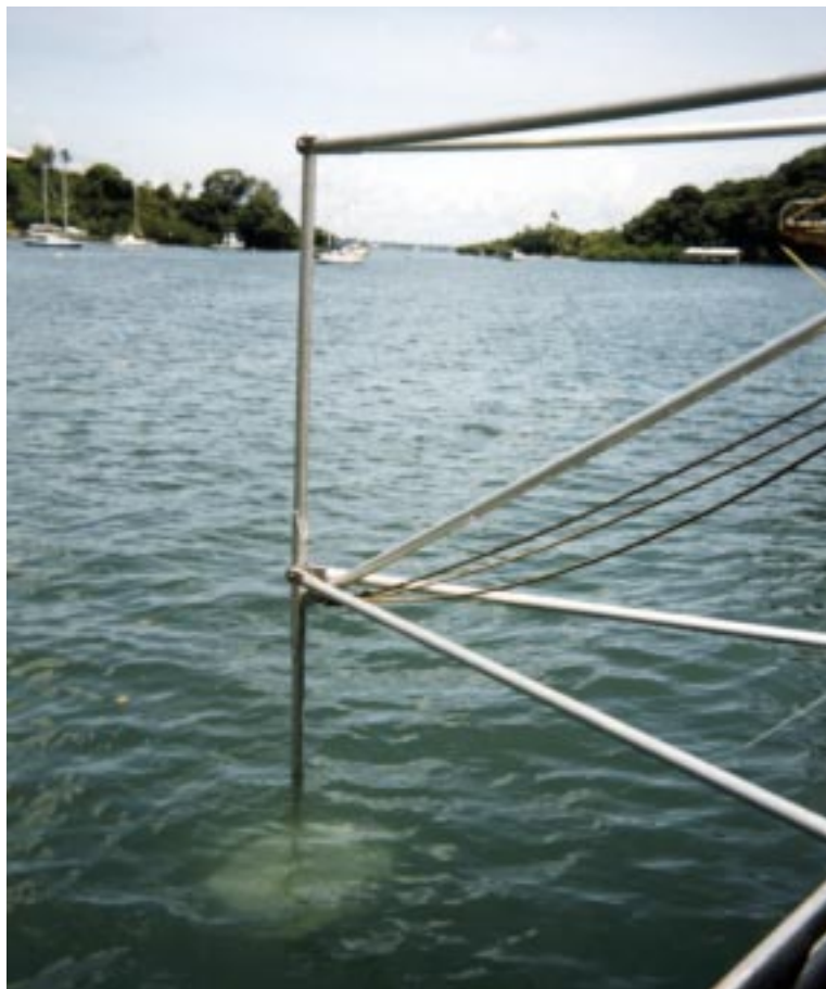
Figure 4: Flopper-stopper being deployed
