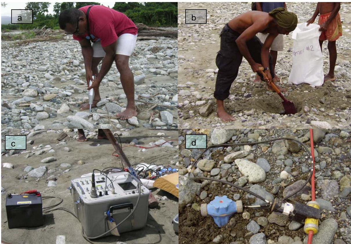
Figure 3. Various methods of aggregate assessment in Waramai and Wara Bili; a) Testing of rock boulder using the Schmidt Hammer. b) Collection of aggregate samples for geotechnical tests. c) The seismograph. d) The geophone clipped to the cable.
