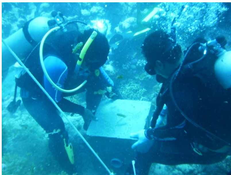
Figure 5 Deployment of temperature loggers in Funafuti, 2011.
