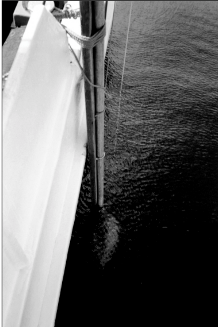
Figure 5: Echo sounder transducer housing mounted on the side of F/V Marwel
