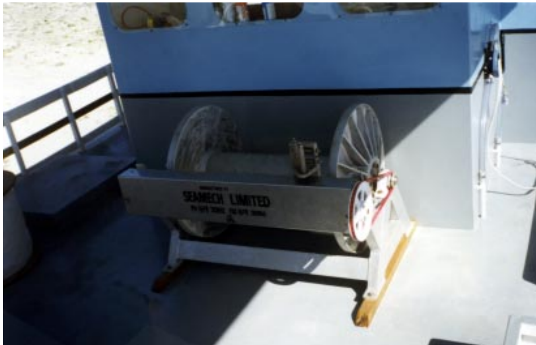
Figure 1: Seamech tuna longline reel mounted on F/V Tekokona II
