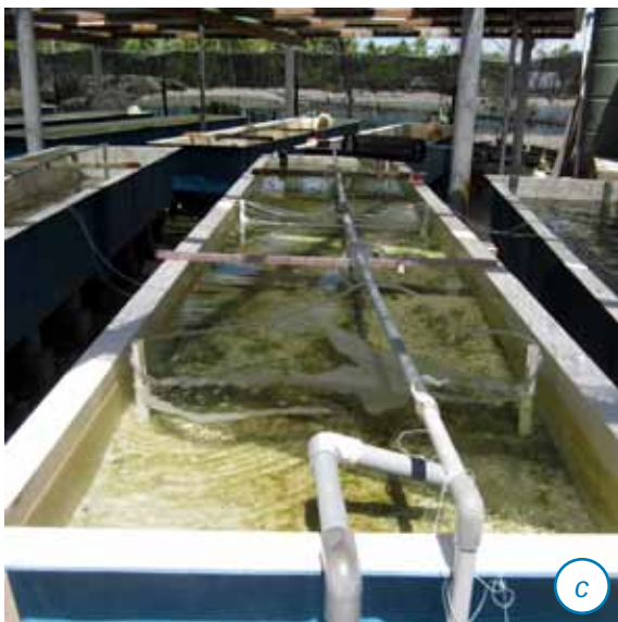
Figure 7. Constructing a habitat simulator tank. Perforated piping and airlift stand pipeset on the tank floor (a); a bottom layer of coral stones (b); coral gravel for the second layer (c); fine sand as a top layer (d).
