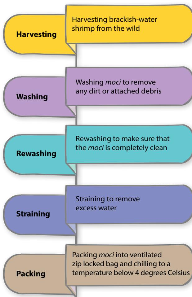
Figure 3. The different steps of the post-harvest process.
