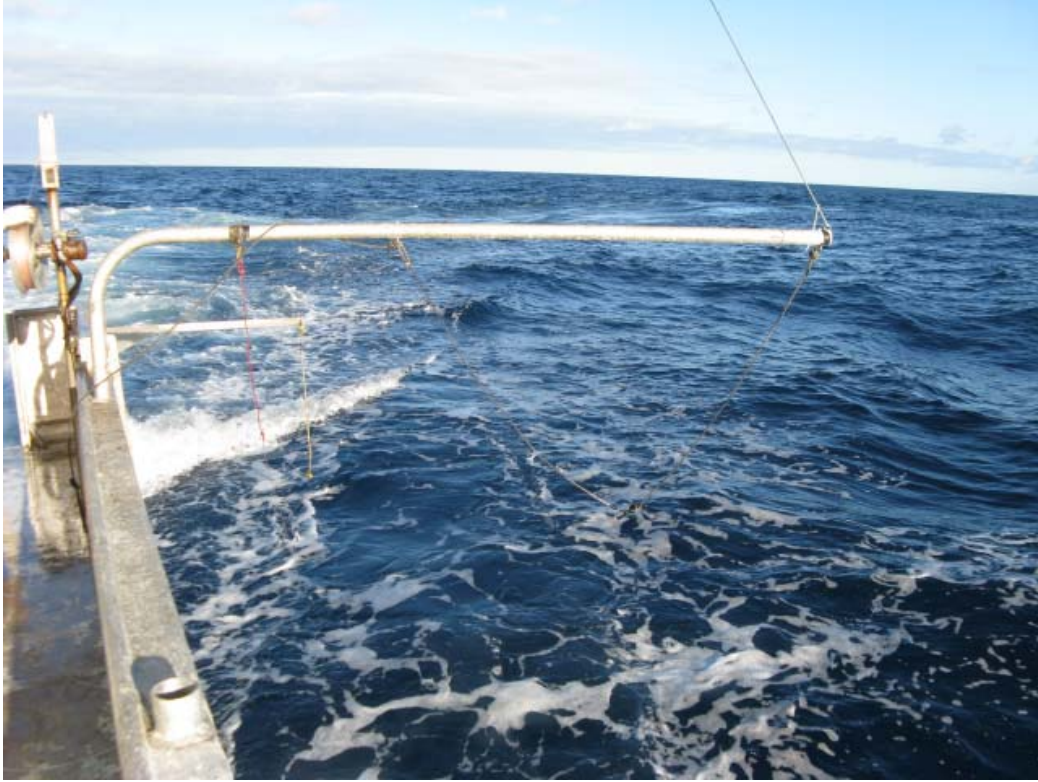
Figure 3. Two dangle poles rigged on the port stern.
