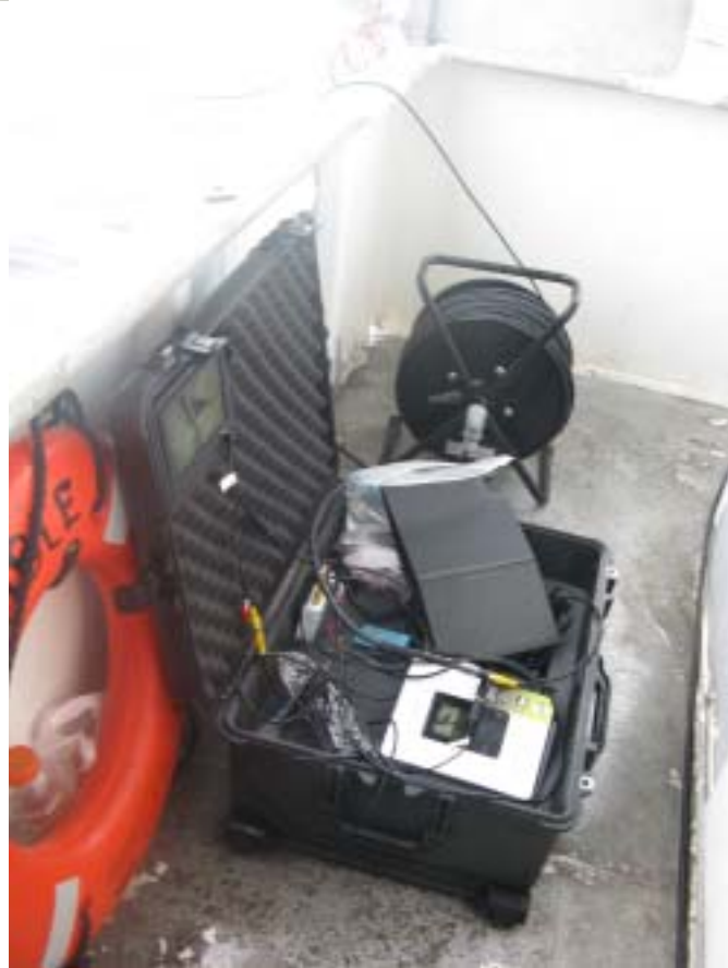
Figure 21. SPLASHCAM system showing video head, stabilizing fin and weight cabled to viewing and recording gear
