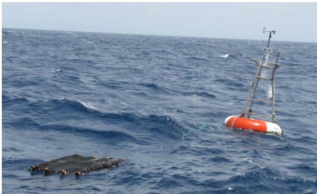
Figure 10. buoy at 5N, 155W with purse seine drifting FAD tied to it and a strobe light on the frame
