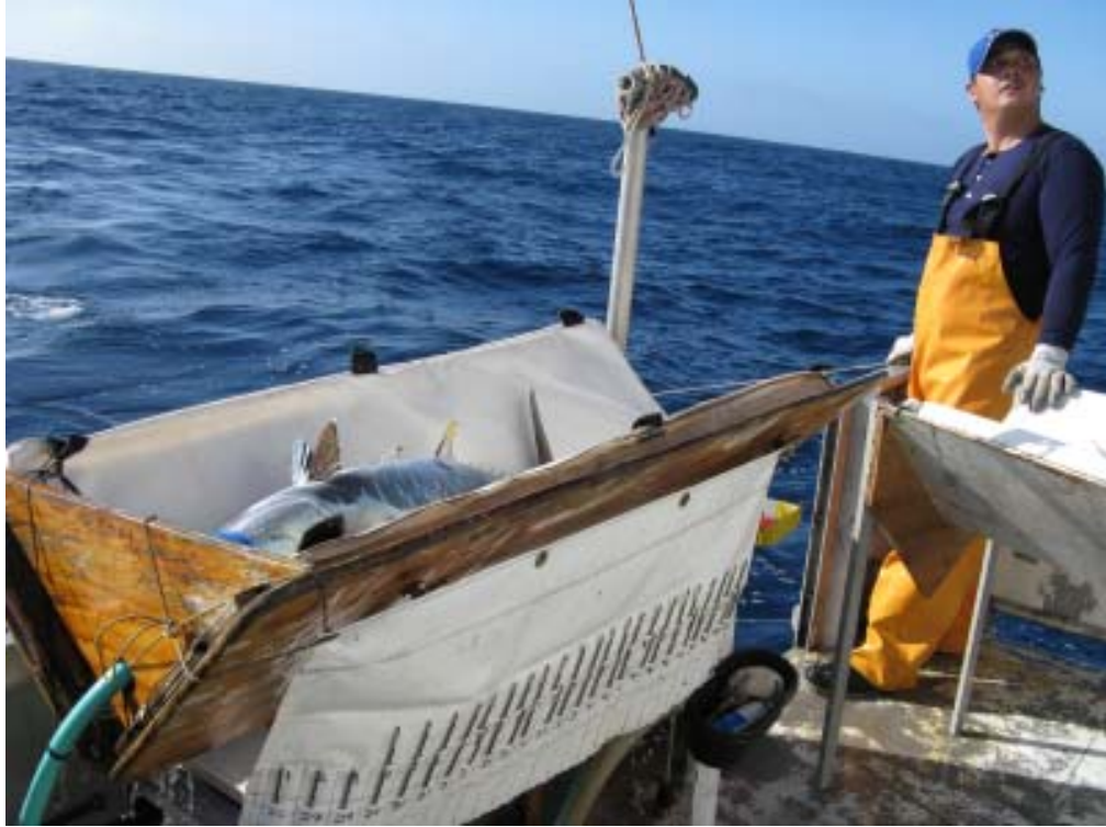
Figure 5. Archival tagging cradle with a tagged bigeye
