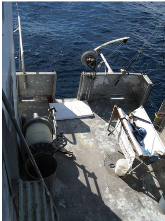
Figure 2. Starboard stern working deck showing one mini-longine reel, one hydraulic trolling reel, a padded tagging mattress and tagging cradle.
