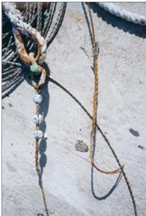
**9.0 mm galvanized wire cable showing splices, one parted**
