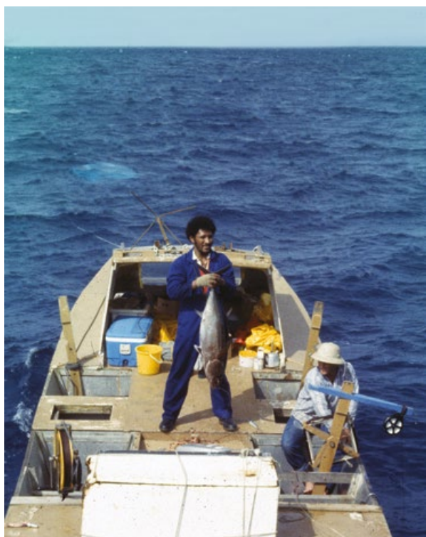
Among other fishing techniques promoted by SPC in the 1980s, the use of the palu-ahi and vertical longlines around FADs allowed to access the bigger deep-swimming tuna. Note the sea anchor used to fish while slowly drifting, facing wind and swell. Fiji, 1984 (image: SPC).
