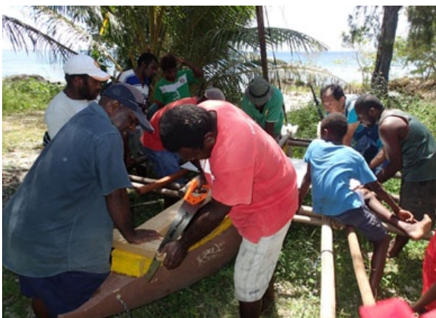
Photo 6. Assisted by the Vanuatu Fisheries Department and a Japanese specialist, local fishermen modify a traditional canoe by equipping it with a sail and small outboard engine. This will help reduce fuel consumption.
