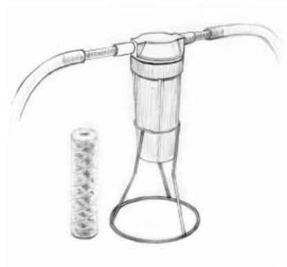
*Fig. 8. Bio-filter (with bio-filter cartridge shown separately)*
