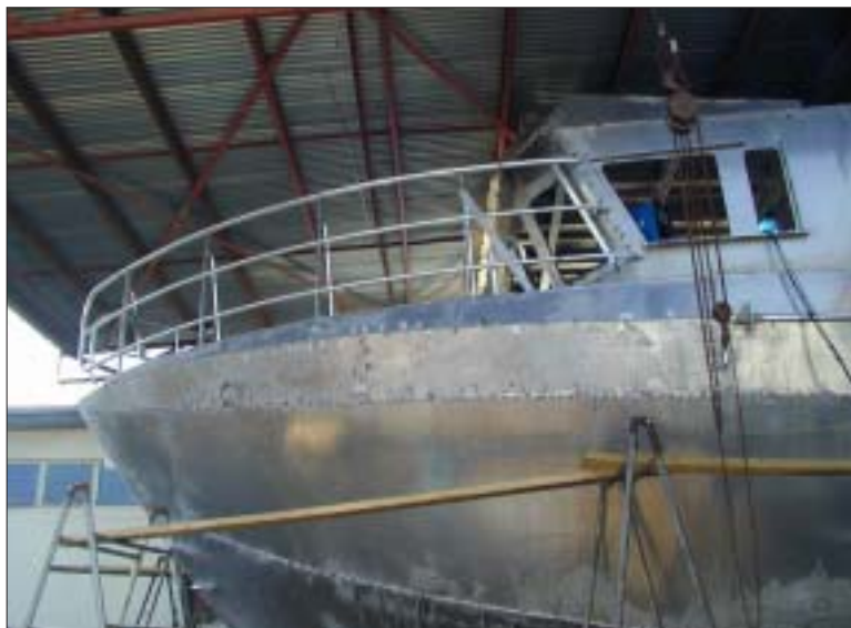
Figure 1: Warren 18 metre longliner under construction
