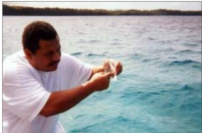
Seaweed specialist, Esaroma Ledua, demonstrates how to check water salinity using a simple field refractometer
