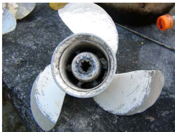
In both incidents, the propeller was the faulty part. This picture of Lonese Natano's propeller was taken after the boat was rescued (image: Semese Alefaio, TFD).
