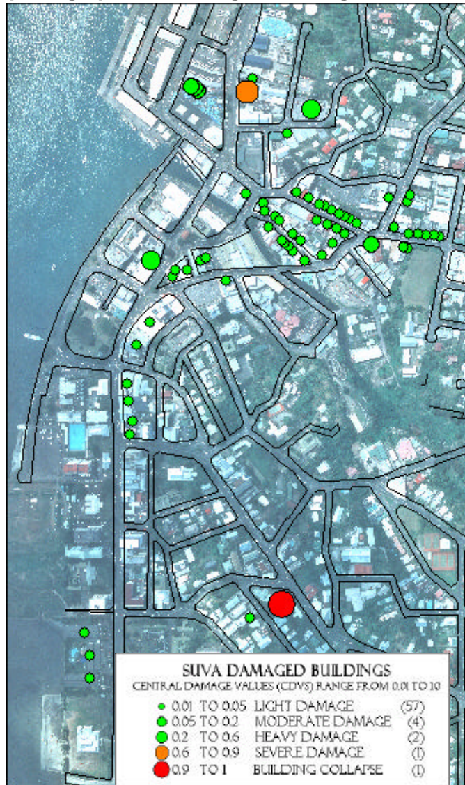
Figure 5b. Suva orthophotograph with damaged buildings assessed and flagged.
