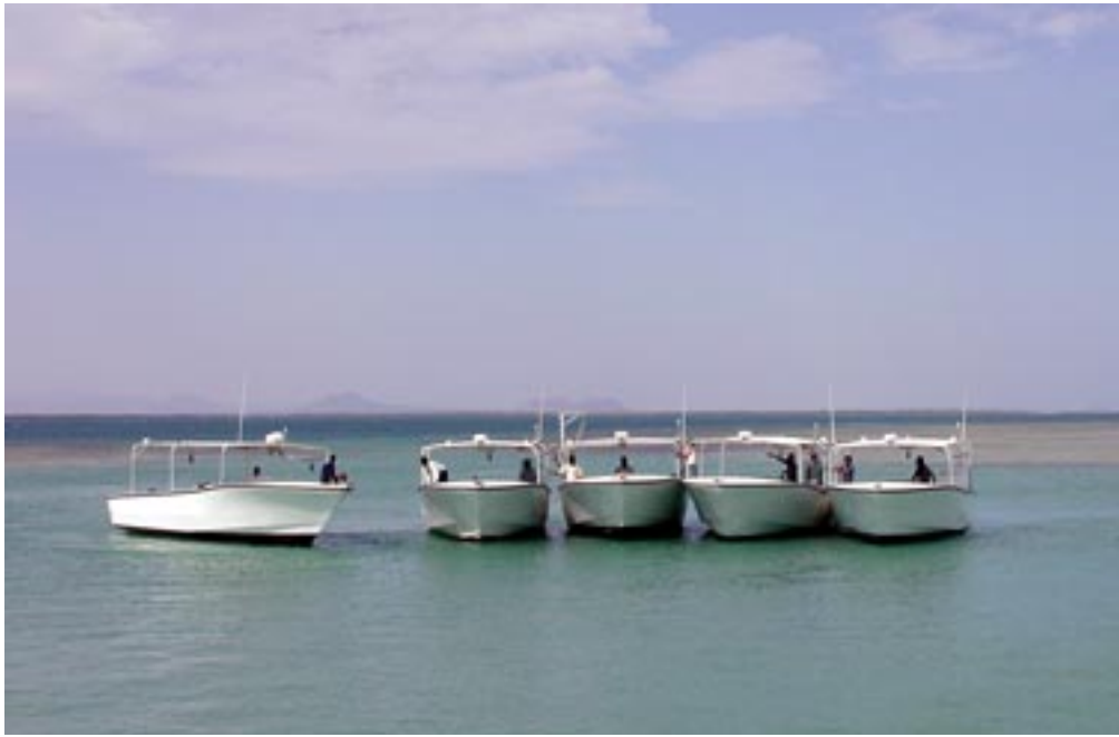
Five new Sea Chrome Marine 11 metre longline boats from the Harena Boat yard on Halib Island, Eritrea. All are equipped with 24" x 27" Lindgren-Pitman monofilament longline reels. They are powered by Volvo-Penta 105 HP sterndrives.
