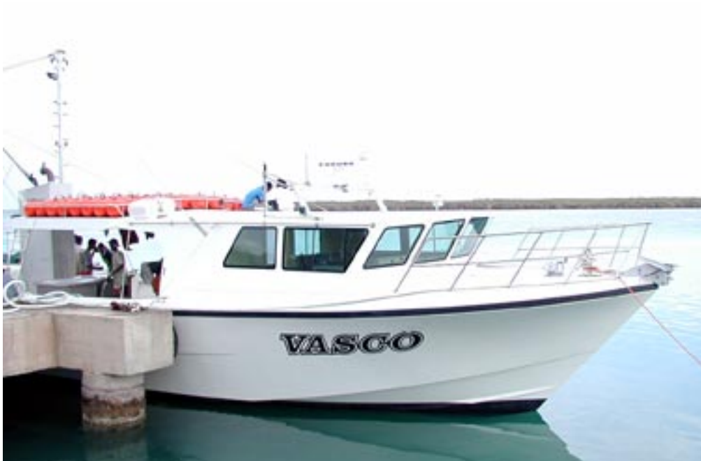
F/V Vasco , the first of many 18 m longliners from Harena Boatyard. Vasco is equipped with a Lindgren-Pitman 38" x 48" Super Spool and an LS-4 Line Setter. The boat is powered by a Caterpillar 3406 diesel.
