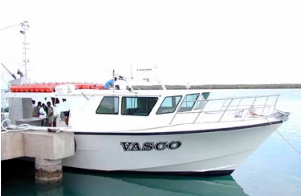
**F/V *Vasco*, the first of many 18 m longliners from Harena Boatyard. *Vasco* is equipped with a Lindgren-Pitman 38" x 48" Super Spool and an LS-4 Line Setter. The boat is powered by a Caterpillar 3406 diesel.**
