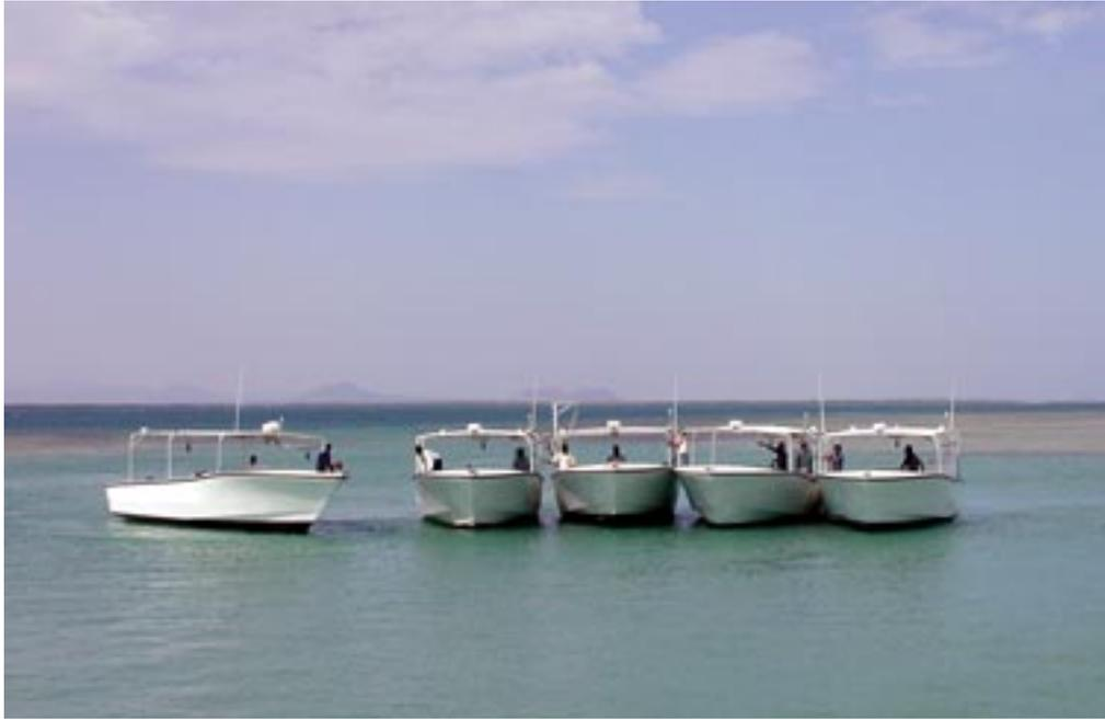
**Five new Sea Chrome Marine 11 metre longline boats from the Harena Boat yard on Halib Island, Eritrea. All are equipped with 24" x 27" Lindgren-Pitman monofilament longline reels. They are powered by Volvo-Penta 105 HP sterndrives.**
