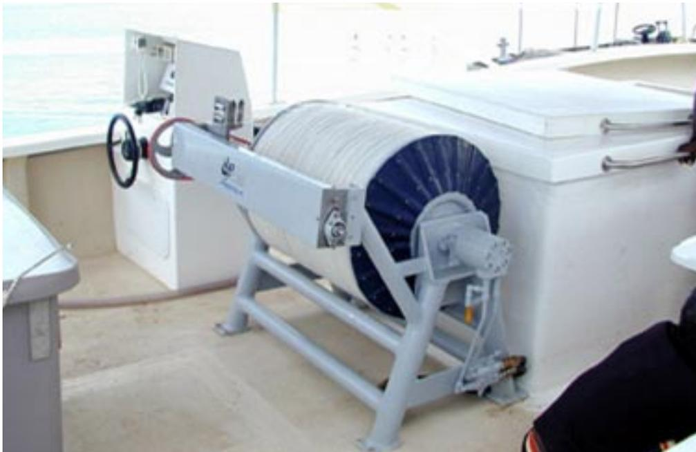
**An 11 m longliner, showing placement of the Lindgren-Pitman 24" x 27" longline reel, and the control station. The insulated fish box is just forward of the reel and a branchline bin is secured in chocks just aft of the reel.**
