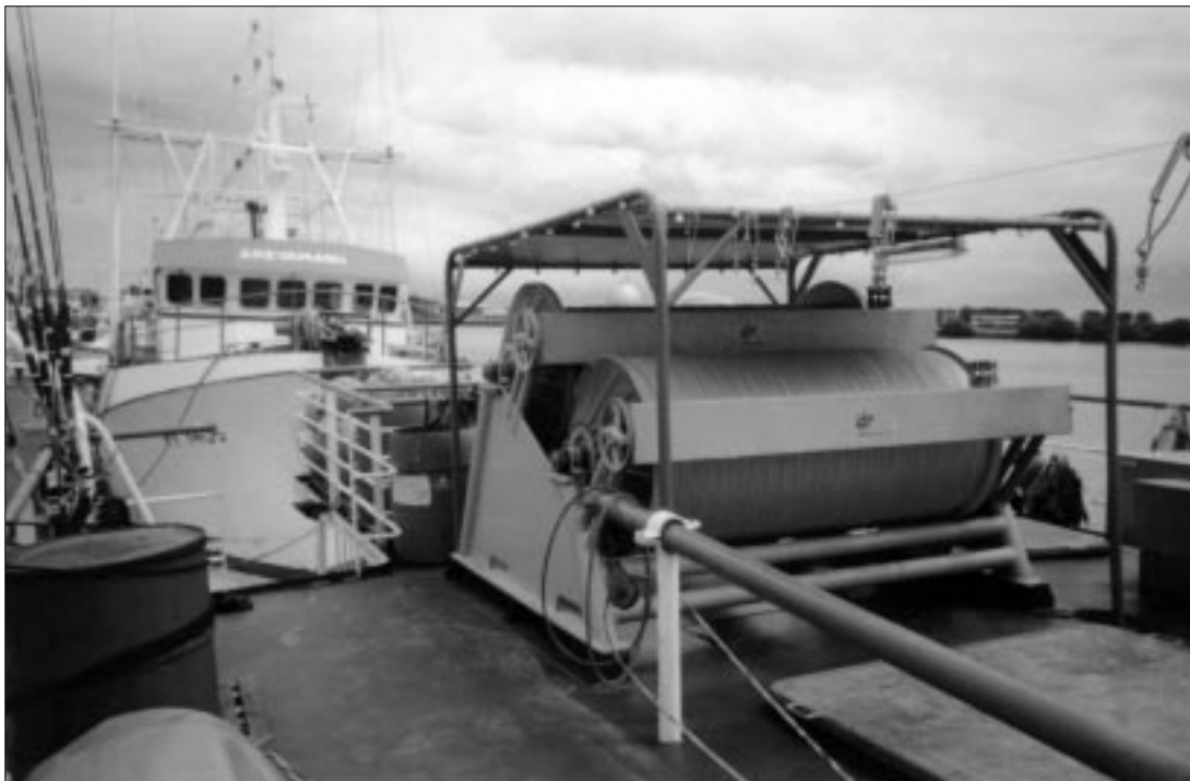
Figure 4: Twin reels on F/V Vini Vini VI
