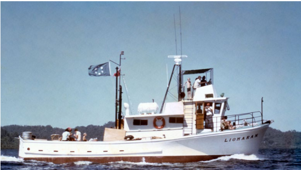
Liomaran , a 16.2 m ferro-cement fishing vessel built in 1974 for the Yap District Office of the Marine Resources Division of the Trust Territory undergoing sea trials at Tulagi, Solomon Islands (image: M. McCoy).
