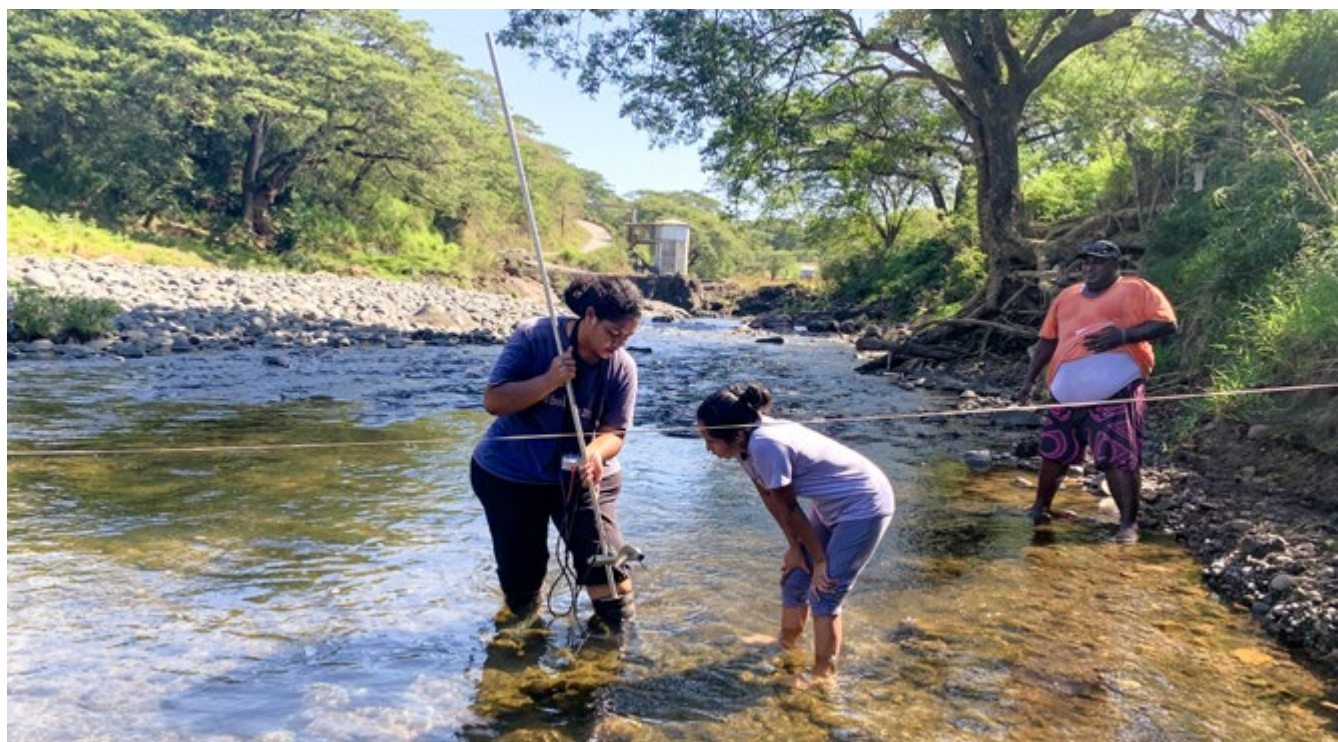
Stream gauging by Fiji Meteorological Service, Fiji, 2022 © Pacific Community (SPC) / Credit: SPC
