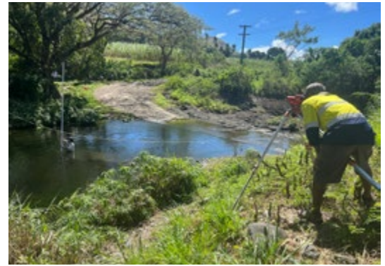
Water Authority Fiji and SPC undertaking a river cross-section survey of Penang River, Fiji © Pacific Community (SPC) / Credit: SPC
