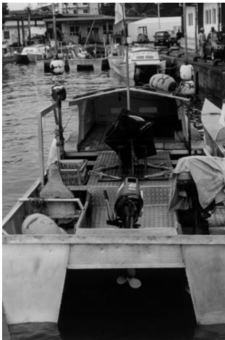
Figure 11: Steel hand-crank reel lashed in the hauling position with frame for pulley mounted on the gunwale
