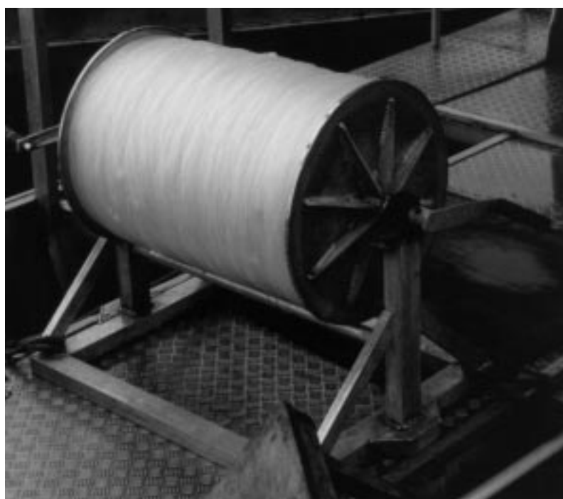
Figure 10: Longline reel constructed from aluminium with a hand-crank on both ends
