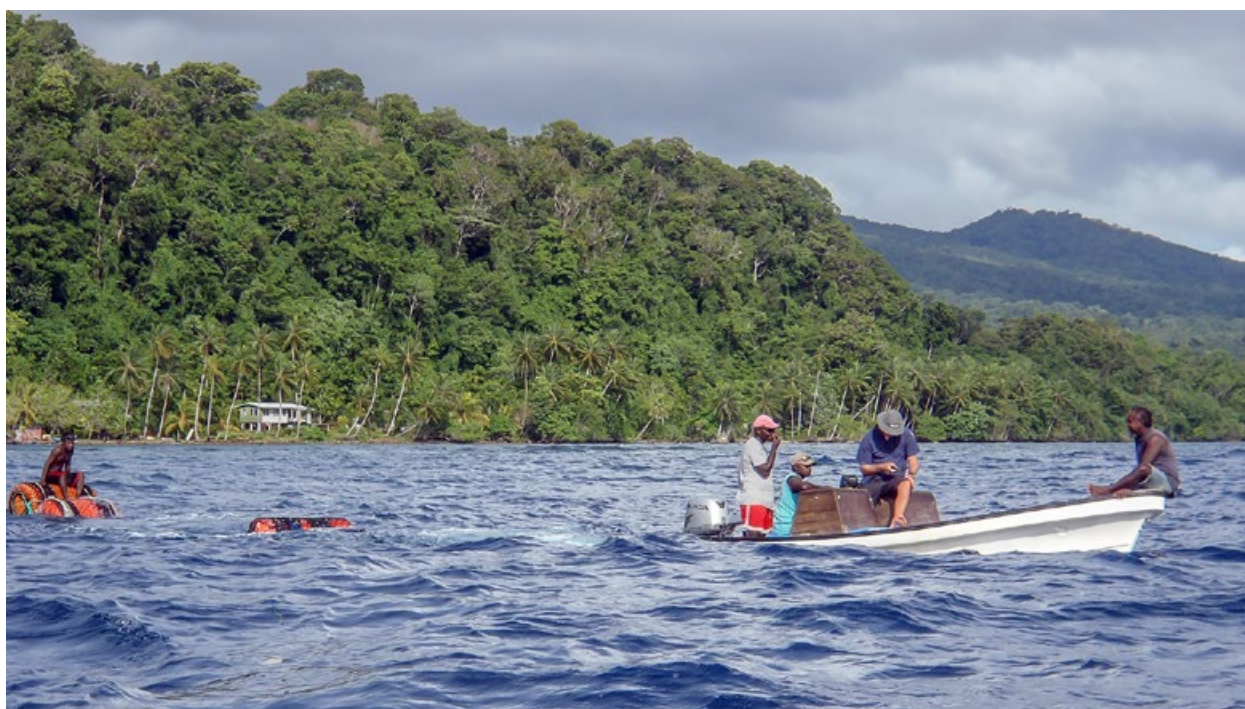
To reduce fish aggregating device cost, the feasibility of setting mid- to shallow water FADs from small crafts was assessed – Solomon Islands, 2011 (image: William Sokimi).
