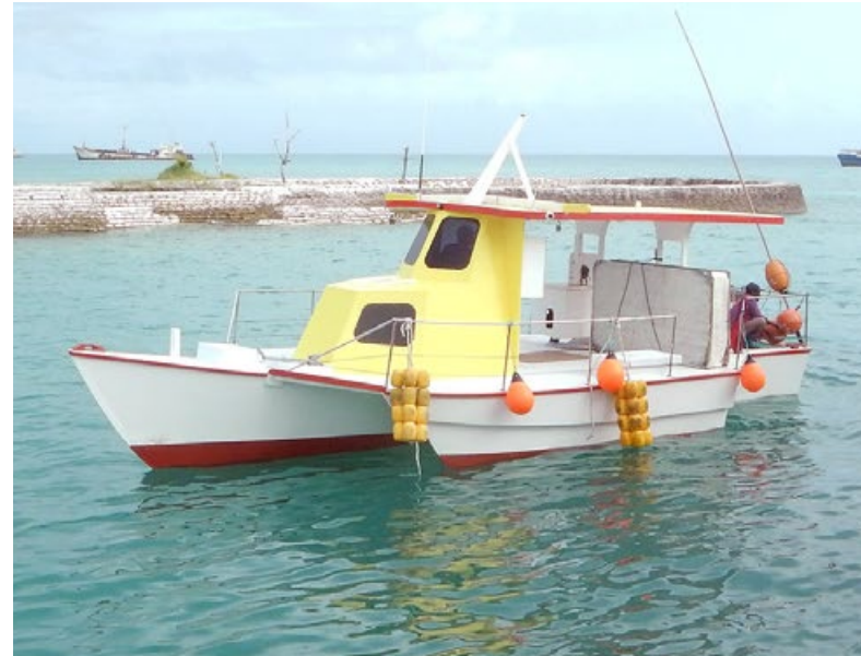
KIR 26 design fishing vessel, a 10.5 m trimaran.
