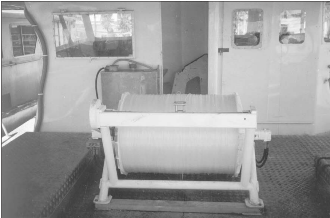
Figure 12: Initial longline reel used on the project vessel
