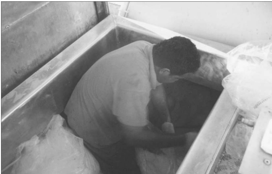
Figure 7: Fish hold with aluminium lining for ease of cleaning
