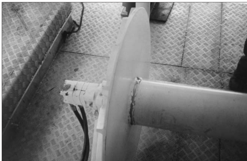
Figure 13: Broken weld and side of mainline reel pushed out
