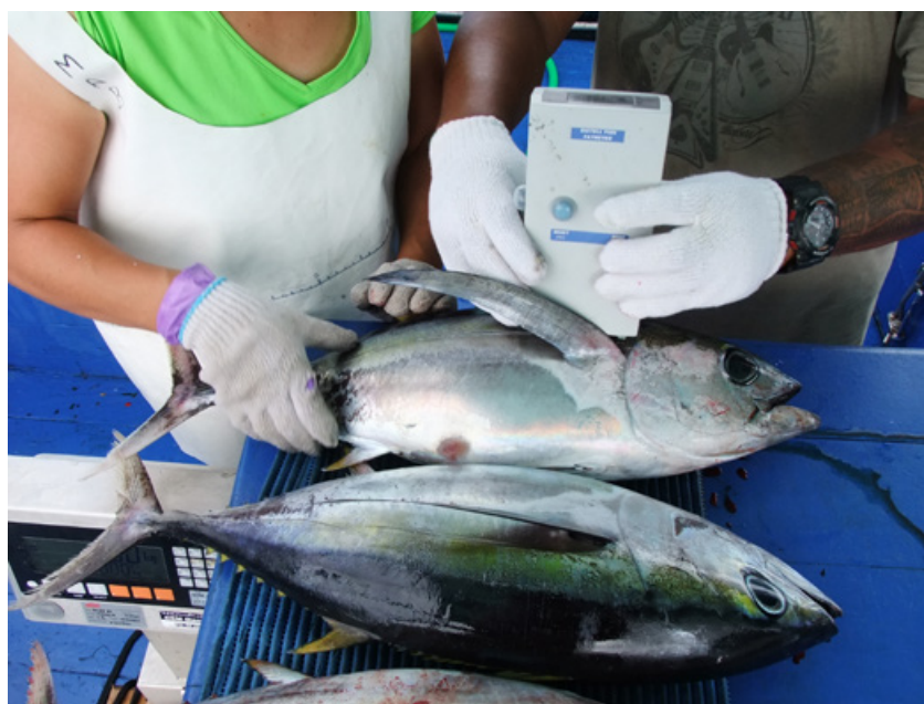
Figure 5. Using a fat meter to measure the fat content of bigeye tuna.
