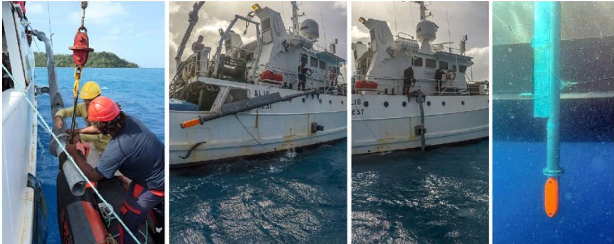
Figure 3. A surface echo sounder is mounted on the side of the RV Alis to observe organisms in the first 10 meters below the surface. Images: Valérie Allain
