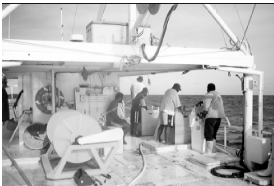
Figure 15: Hauling arrangement with unsnapping position forward of steering console
