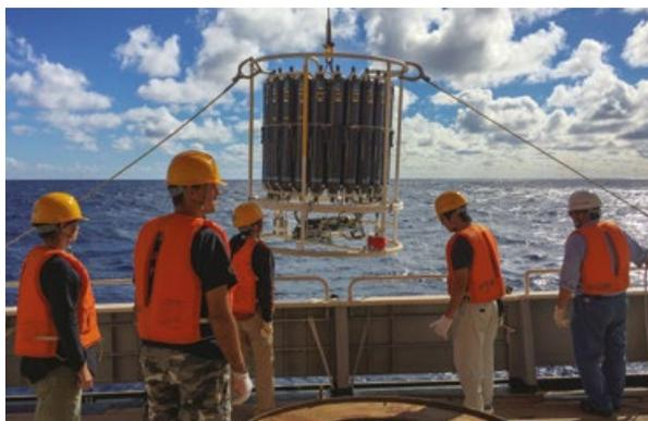
Gear used to collect and analyse seawater's physical and chemical characteristics, from 0–1000 m depths (image: Élodie Vourey).
