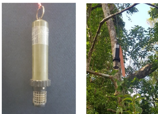
Figure 3-1 : A New Zealand Department of Conservation-made ABM used for monitoring bat calls (left) and mounted in a tree (right)
