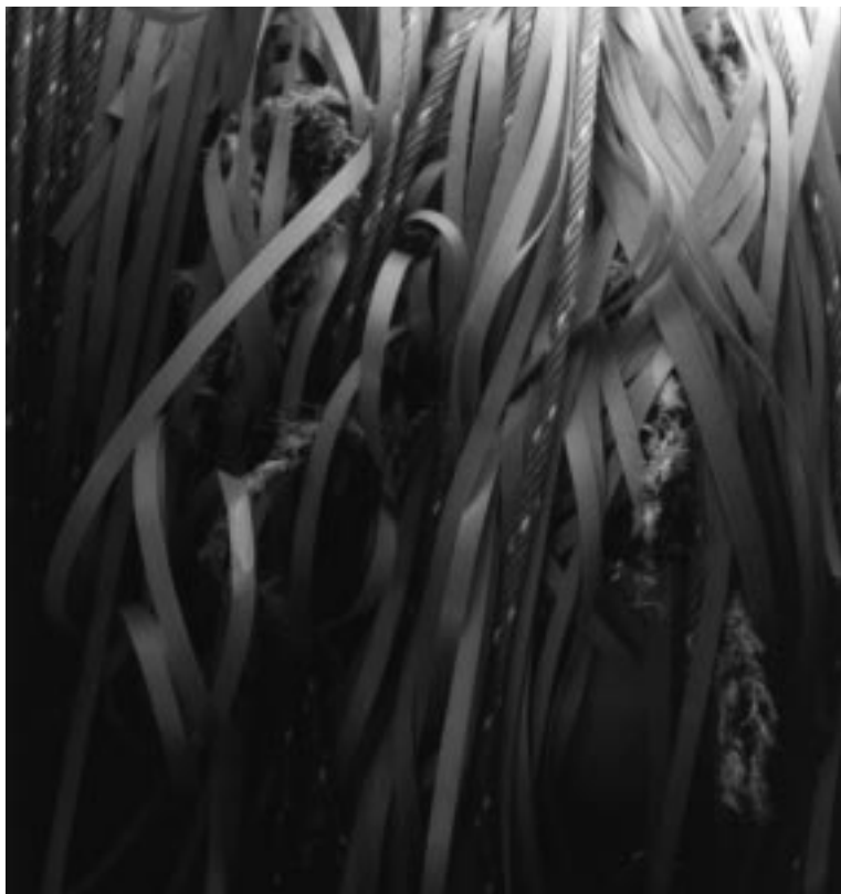
Figure 5: Combination rope used for mooring line with streamers on the top section and pressure floats attached to the middle section
