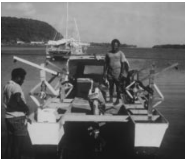
Figure 1: Plywood Alia catamaran with outriggers and four handreels used for trolling (1983)
