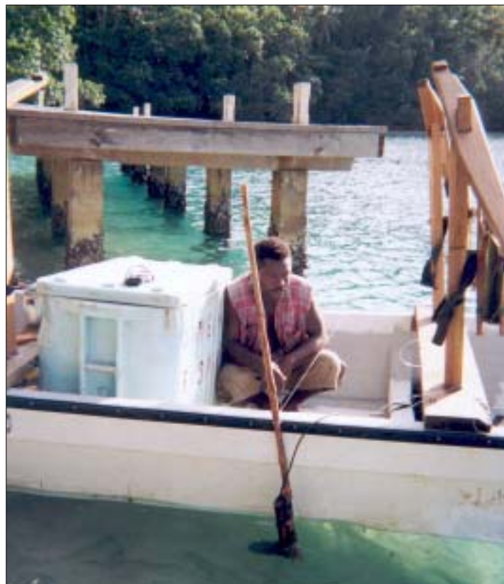
Figure 2 (top): Mounting and power supply for the project echo sounder
