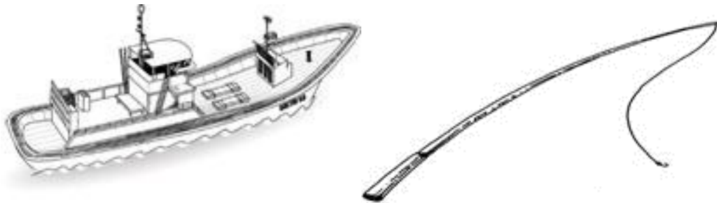
Figure 3.2 Pole-and-line vessel and gear
