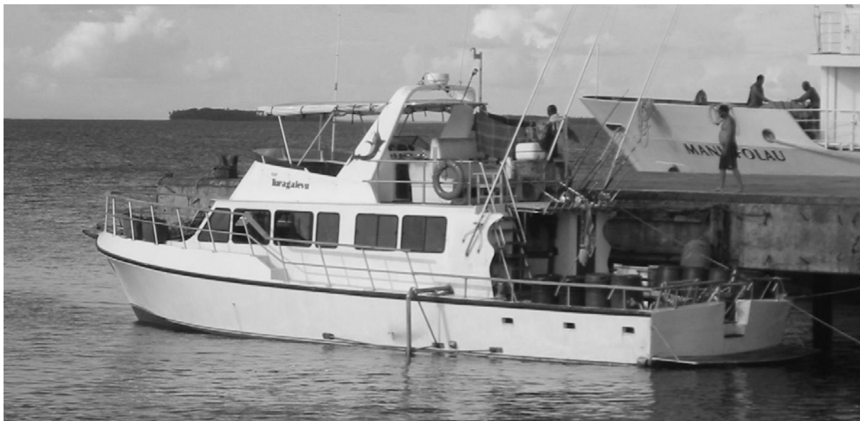
Figure 9. The chartered survey vessel Turagalevu. Note the portside pole mount with fore and aft stabilisers.
