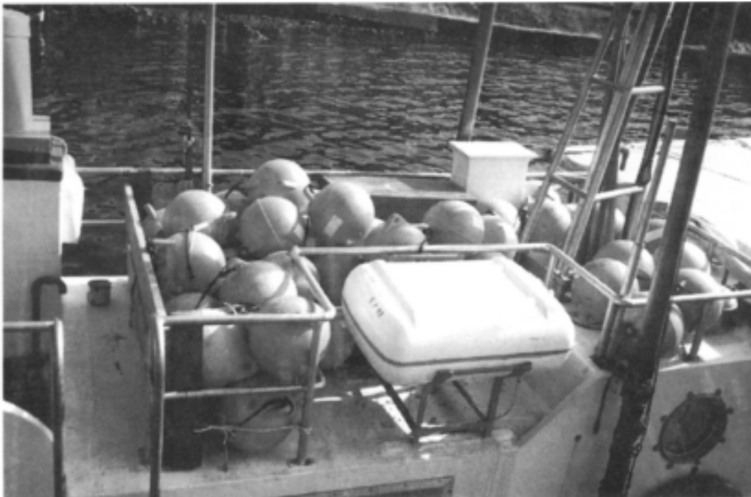
Figure 27: Floats stored on top of the cabin just aft of the wheelhouse
