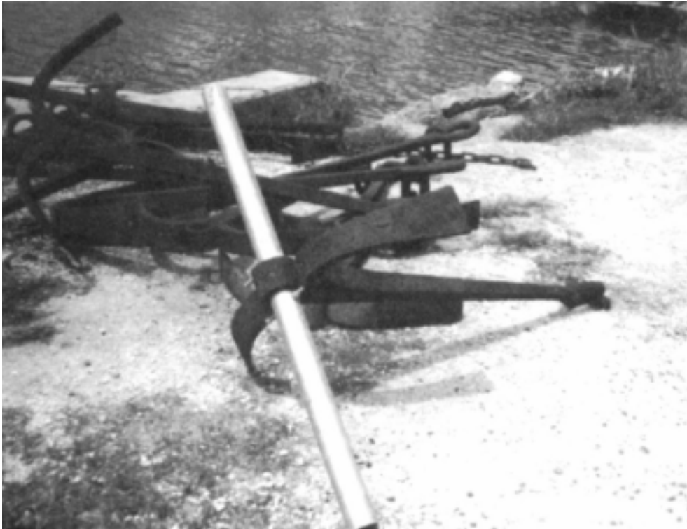
Figure 10: Recovered kedge-type anchors with pipe inserted in crown
