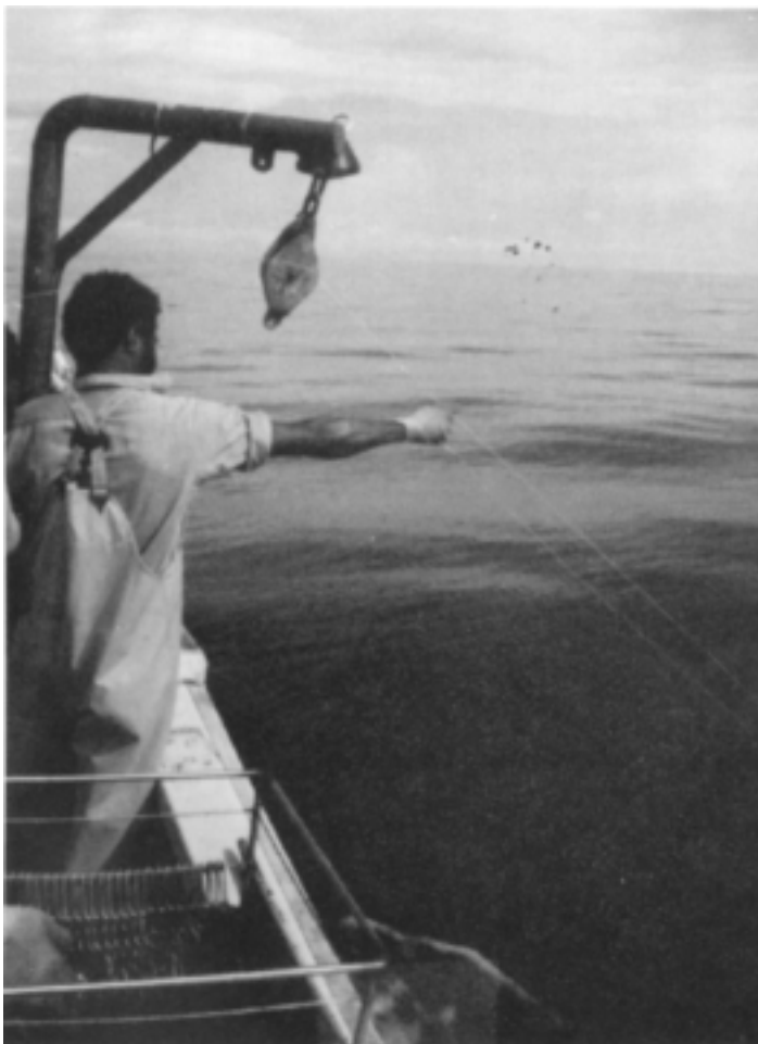
Figure 34: Roller man operating the control valve for the reel and unsnapping the branchlines from the mainline
