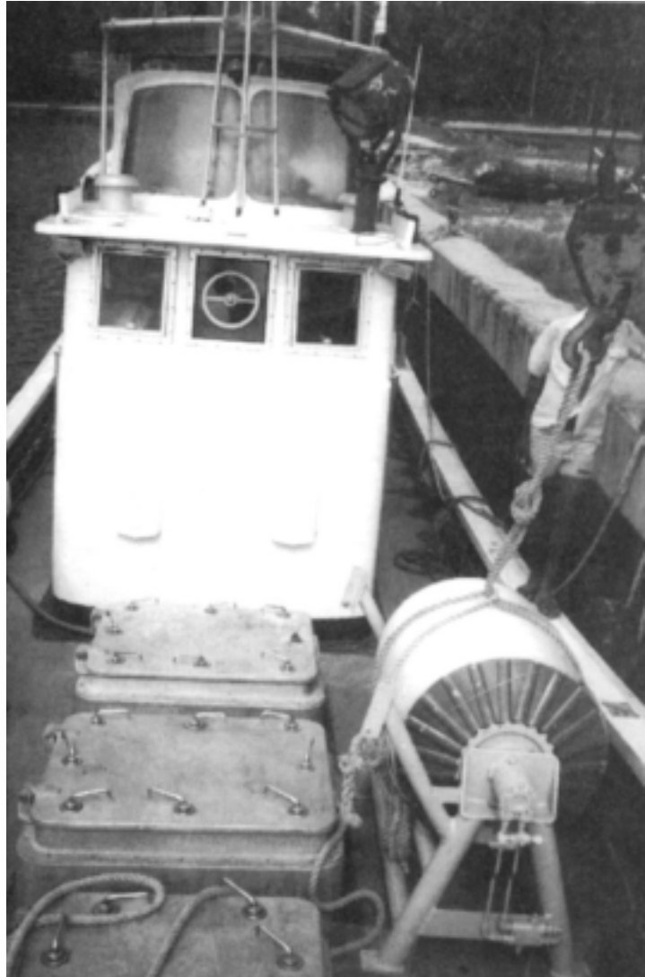
Figure 20: F/V Kuriap listing with the reel sitting on the port side
