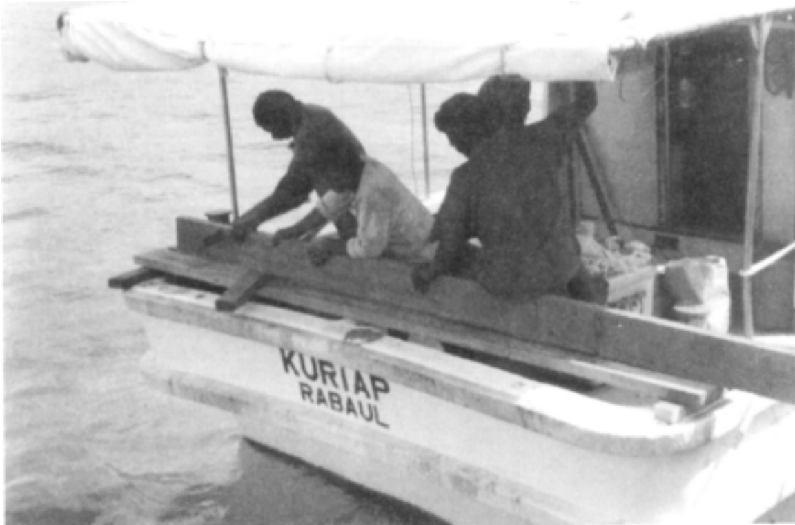
Figure 14: Wooden bench fitted at the stern of F/V Kuriap
