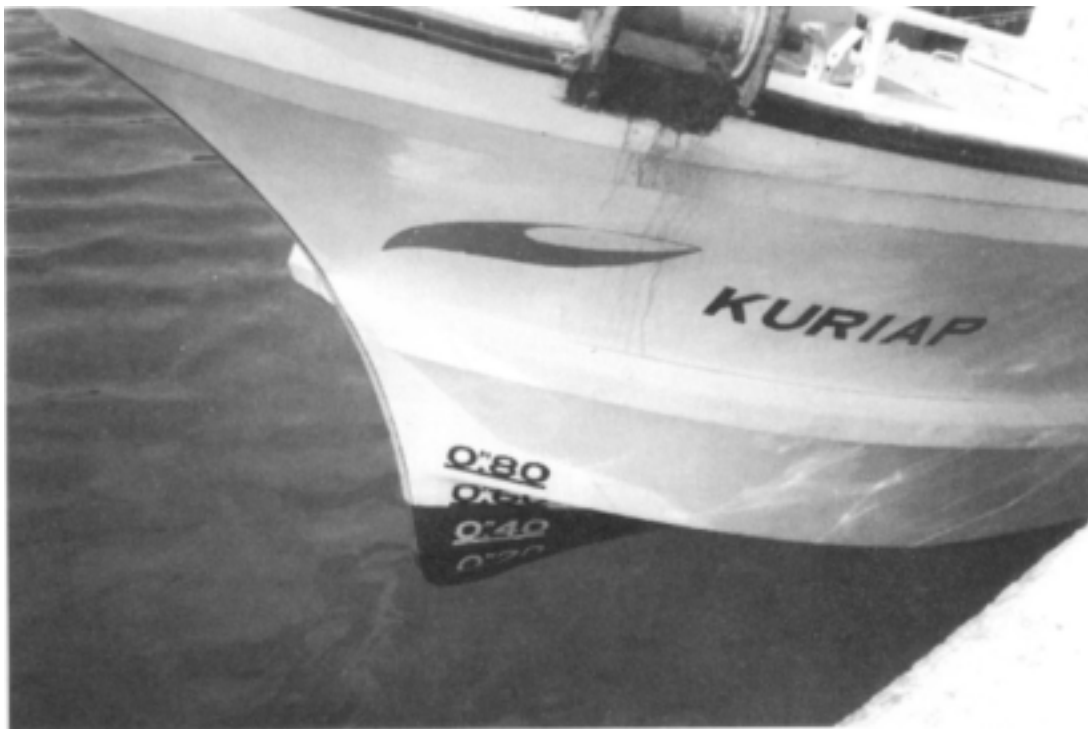
Figure 22: F/V Kuriap 's load line was not affected by the reel's positioning
