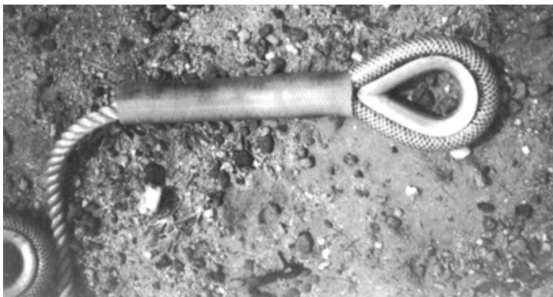
Figure 9: Eye splice in rope, with thimble and PVC covering
