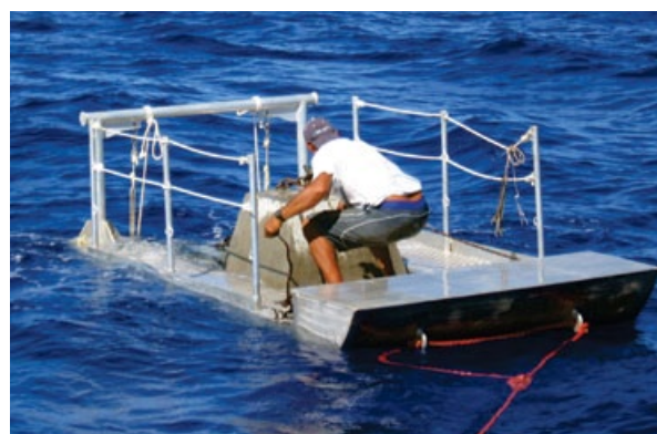
Figure 10. Barge used in Tahiti to carry the cement block anchor.
