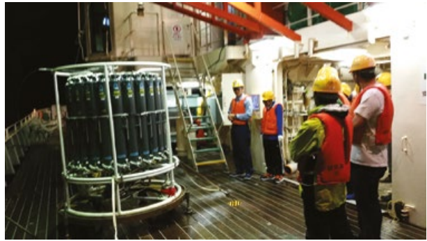
Work on deck to deploy the sampling gear continued day and night. This is the CTD with Niskin bottles, about to be lowered to 1000 m depth.
